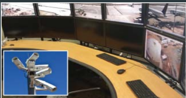
This “virtual tower” uses cameras and monitors to simulate a physical observation ramp tower.
